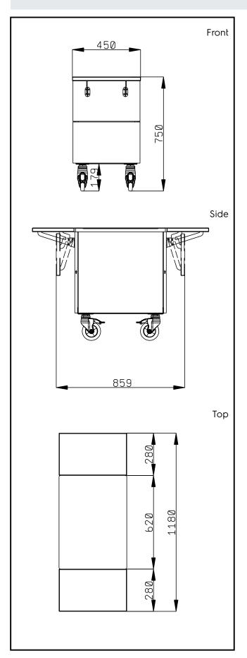
Flexy Compact Ambient unit on cupboard (1GN) with wheels, H=750mm
